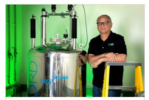
Salk Professor Joseph Noel, pictured in his lab, next to an NMR spectroscopy machine, which is used to decipher the detail of the electronic structures of molecules.
